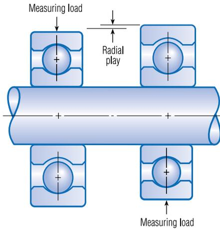
**Fig. 3.** Radial play is a measure of internal clearance and is influenced by measuring load and installation practices. A high radial play value is not an indication of lower quality or less precision.
