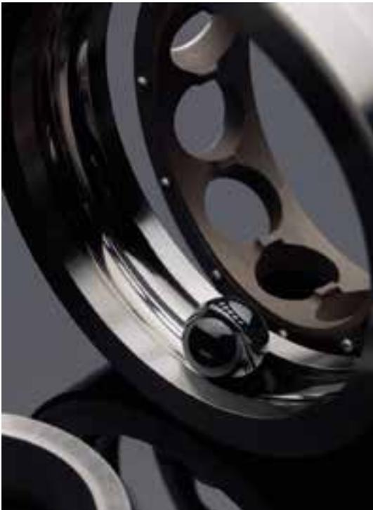
Barden super precision bearings come in inch or metric dimensions with diameters ranging from 4mm ( $\frac{5}{32}$ " OD) up to 300mm (11½" OD). A variety of seals, shields and metallic/non-metallic cage designs are available to meet most requirements. Many Barden bearings operate comfortably at speeds reaching 2 million dN (bore in mm x RPM), or above.
