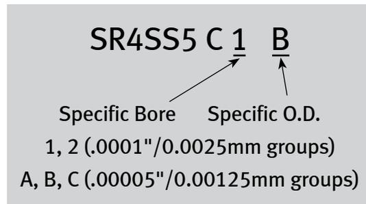
**Fig. 24.** This drawing, grossly exaggerated for clarity, illustrates specific calibration options (inch) for bore and O.D.
