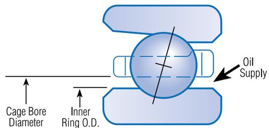
■ Fig. 17. Lubrication window for B-type bearings.
