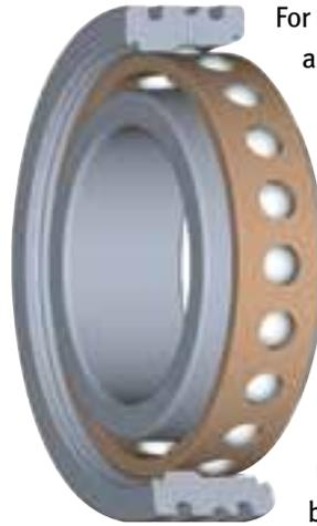
For high speed oil lubricated applications, many bearing types can be supplied with radial lubrication holes to take oil in close proximity to the ball to raceway contact zones from the bearing OD. The number and size of the lubricating holes can be varied to suit each application, and these holes are connected by a radial oil distribution groove. O-rings on either side
