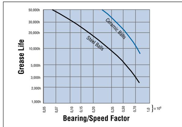
The use of ceramic balls significantly increases bearing grease life performance.
